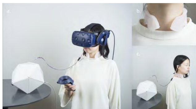
Figure 1. (a) A user wearing a Biometric Visceral Interface and navigating in a computer-mediated virtual space. (b) A soft robot actuator on a user's neck. (c) A haptic link between the user and the device that incorporates pulse sensing on the user's ear.
